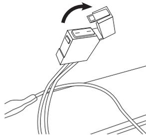
**2** Open fuse box located on the battery.
