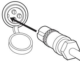
**1** Plug the charger into the port on the Dune Buggy. Make sure the power switch is in the "off" position.
